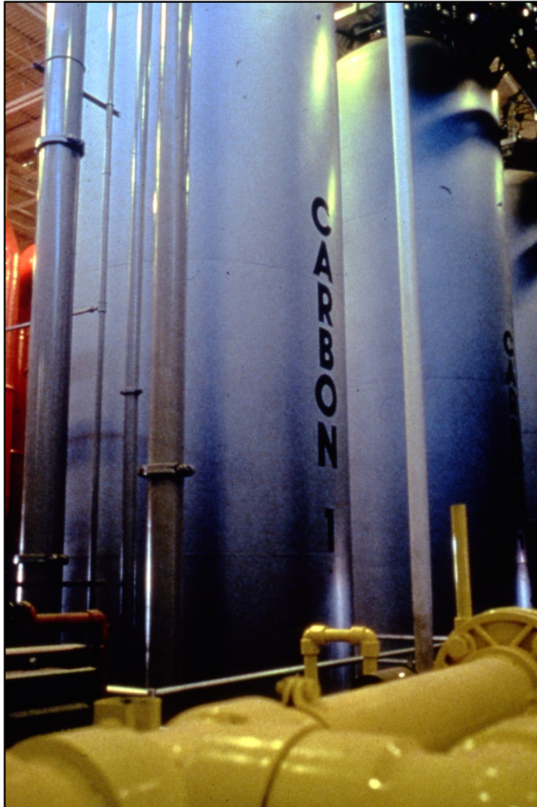
Main Process Area Interior- Carbon Tanks
